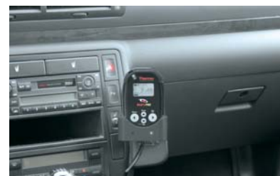
RadEye dash board adapter for mobile area survey applications including optional charging of the batteries
